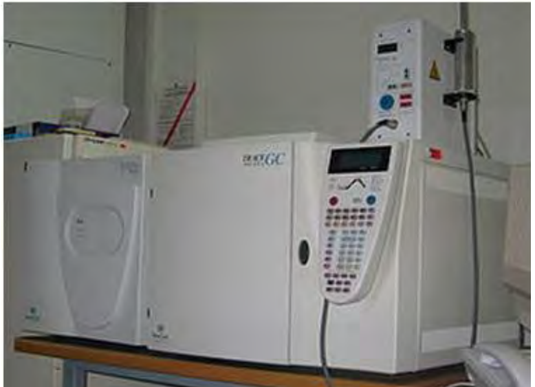
A gas chromatograph (above) directly coupled to a mass spectrometer (below).
