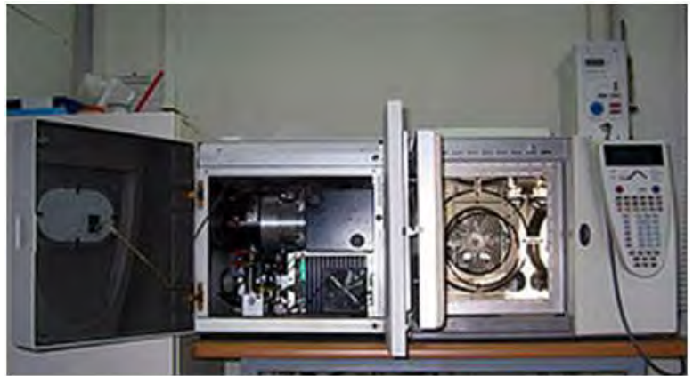
A gas chromatograph (above) directly coupled to a mass spectrometer (below).
