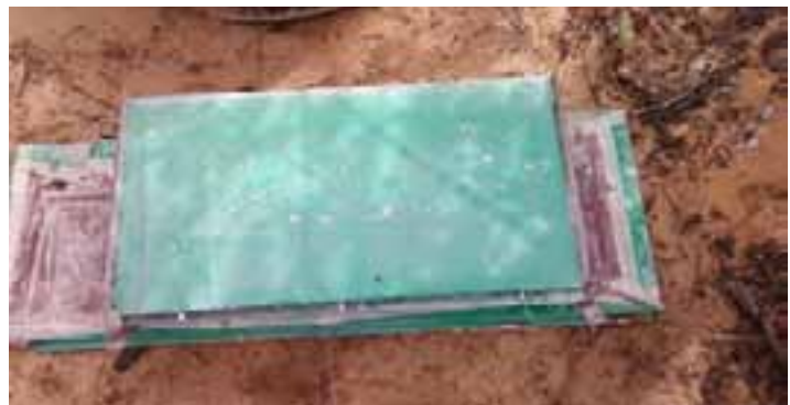
The gabarit is a vinyl coated form used to make a hive.
